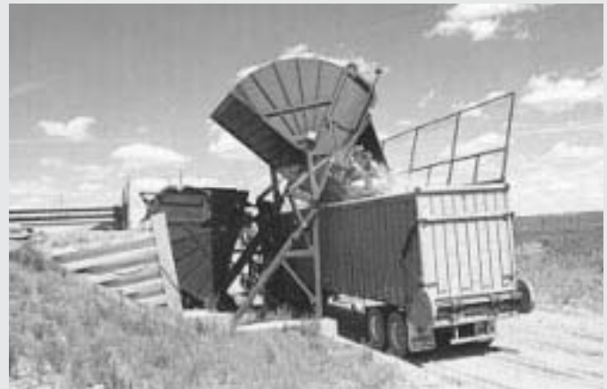
An example of a modular, self-contained waste transfer system. Source: Haul-All Equipment Systems. 1999. Reprinted by permission of Haul-All Equipment Systems.
