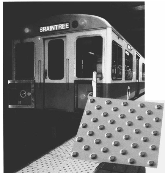
FIG. 5-12. MBTA STATION WITH DETECTABLE WARNING TILE (SUMMITVILLE).
