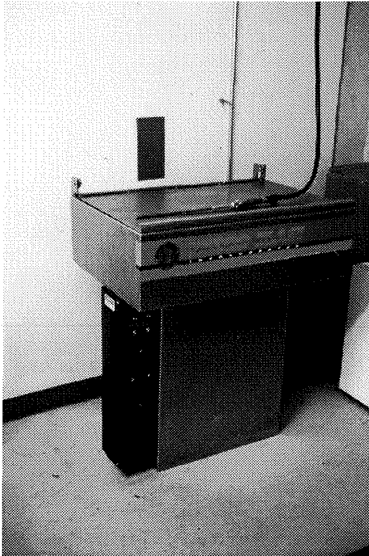
Figure 2-6. Parts Cleaner at Fortner Engineering
