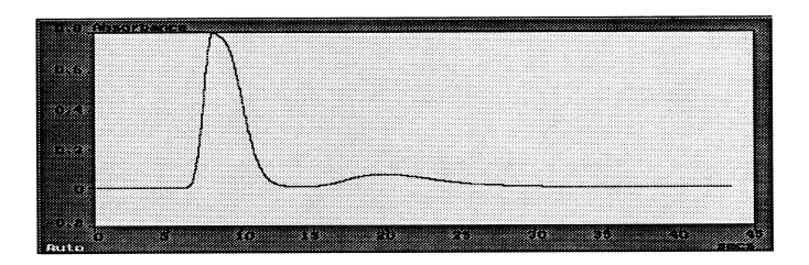
The two individual peaks correspond to the two absorbance cells of different sensitivities. The maximum intensity of the long pathlength cuvette (low range cell) occurs at ~8 sec and the maximum intensity of the short pathlength cuvette (high range cell) occurs at ~20 sec.
