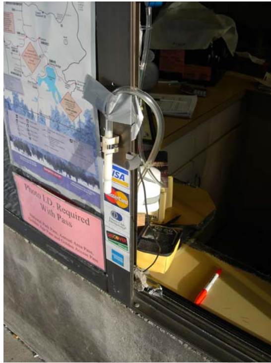
Figure 7. 9mm cyclone in traffic lane of kiosk A
