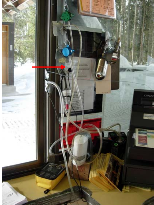
Figure 3. Area sample showing a dosimeter microphone placed at hearing zone level of a gate attendant inside kiosk A (arrow)
