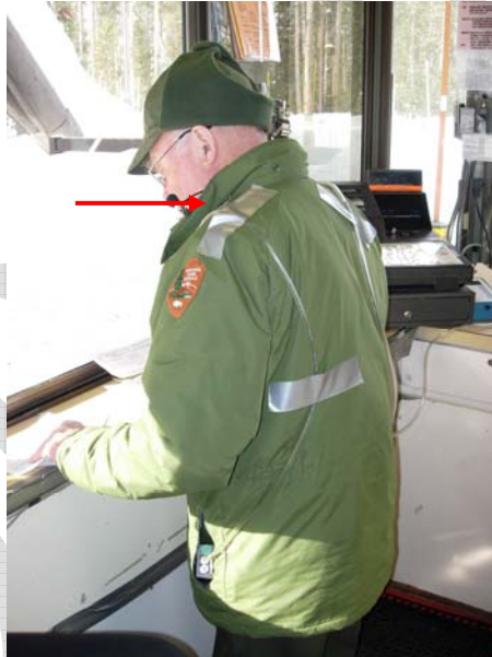
Figure 2. Personal sample placed in the hearing zone of kiosk A gate attendant (arrow)
