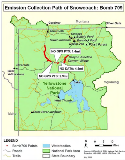
Figure B9. Xanterra Bombardier #709 trip on February 10, 2005. This was a roundtrip from the north entrance to Canyon. This vehicle had two labeled periods where valid data was collected but the GPS was not reporting.
