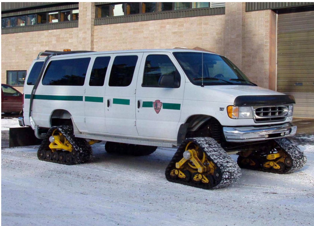
Figure 10. National Park Service 2000 Ford E350 Diesel snowcoach with Mat-trax conversion also showing the insulated exhaust sampling lines.
