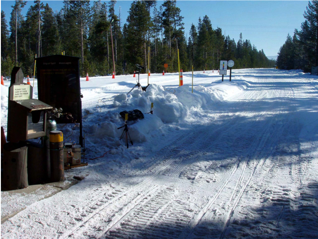
Figure 1. Photograph of the remote sensor, speed sensors and camera setup at the west entrance to Yellowstone National Park.
