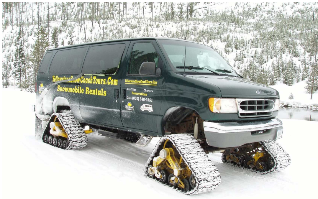
Figure 7. A 2000 Ford Van with a 4 wheel drive Mat-trax conversion. Visible is the exhaust sampling line.
