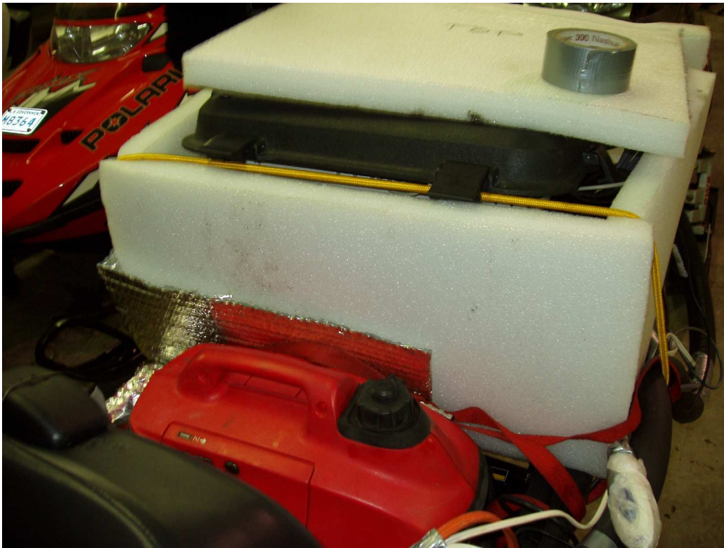
Figure 15. Insulated clam-shell chest with the Montana unit inside with the generator wedged behind the back seat of the Arctic Cat snowmobile.
