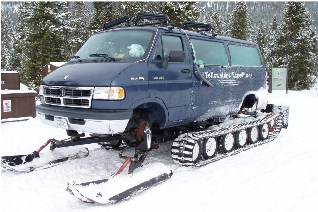
Figure 5. A 1994 Dodge Van with a rear driven Snowbuster track/ski conversion. Visible are the exhaust exit line and the engine diagnostic data cable.
