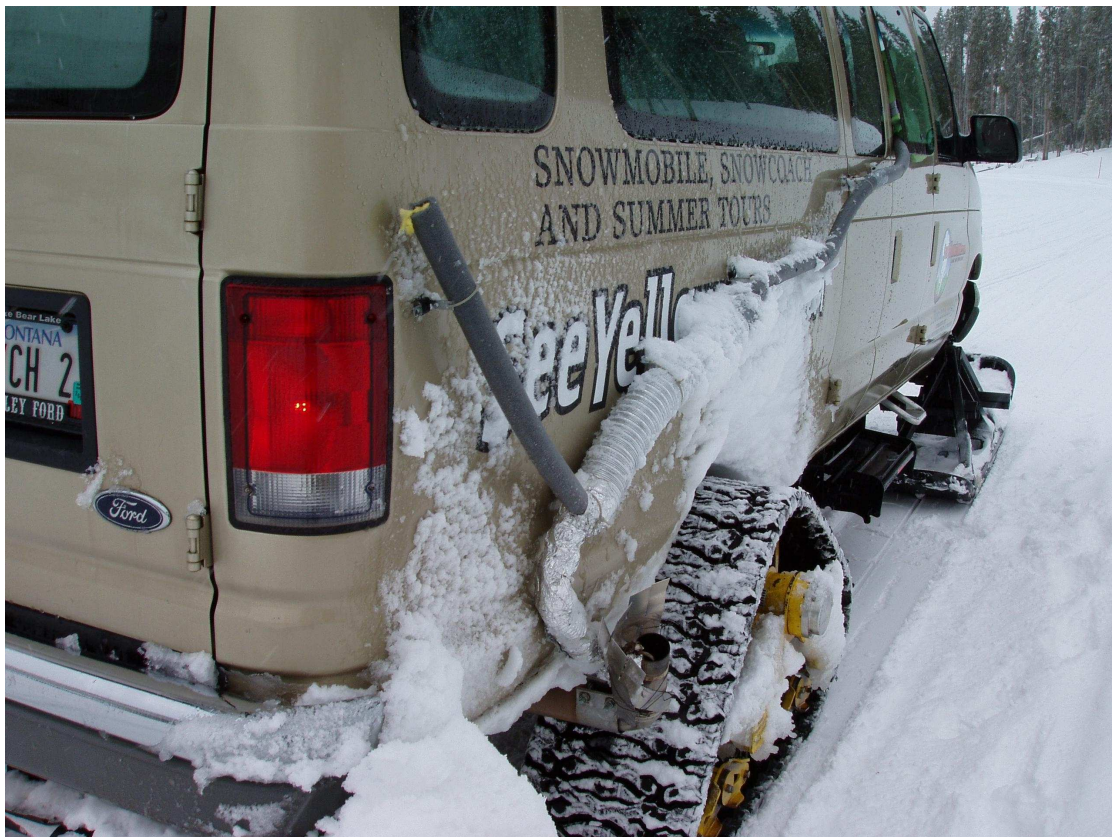
Figure 10. Rear view of a coach showing the tailpipe extension, insulated sample line and the temporary foam insulation installed to seal the side window.
