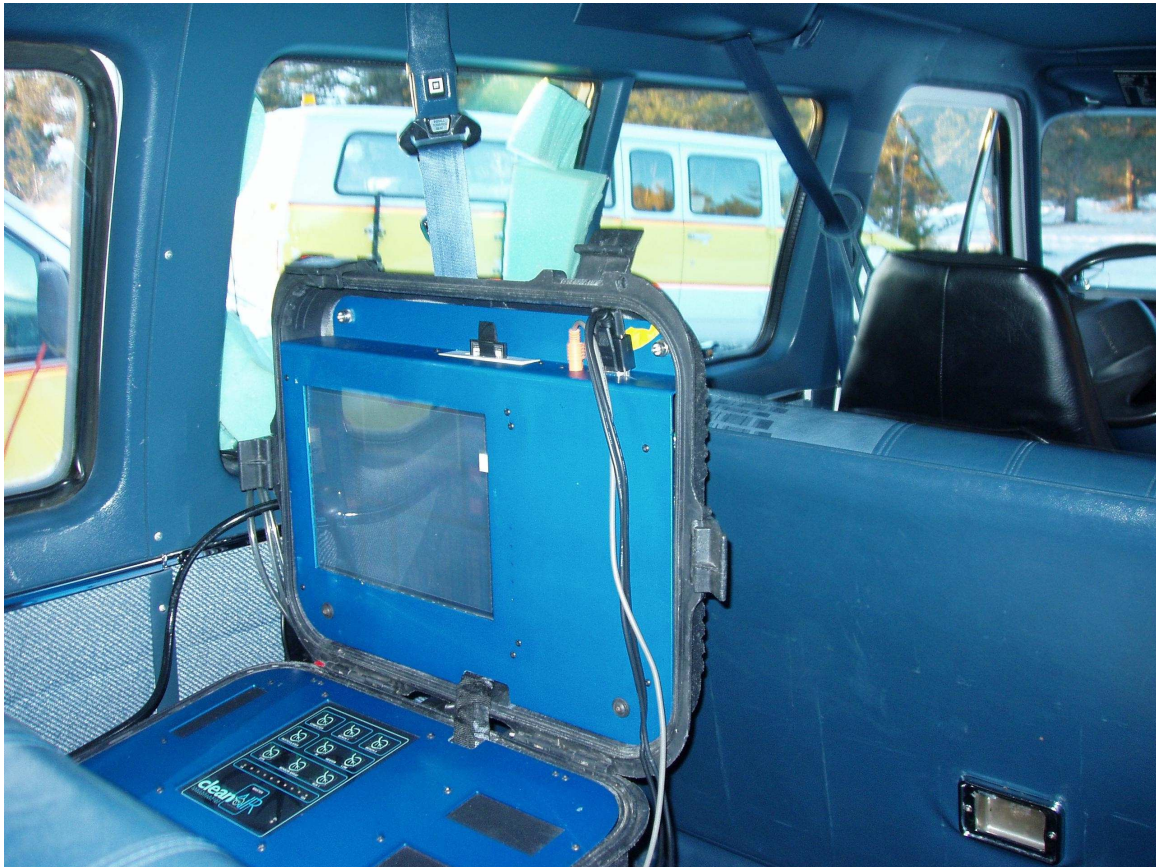
Figure 1. Photograph of the Montana system ready for sampling in a coach. Pictured are the video screen at left, compact flash card top center, GPS receiver connector top right and the exhaust lines exiting the cabin through the side window.
