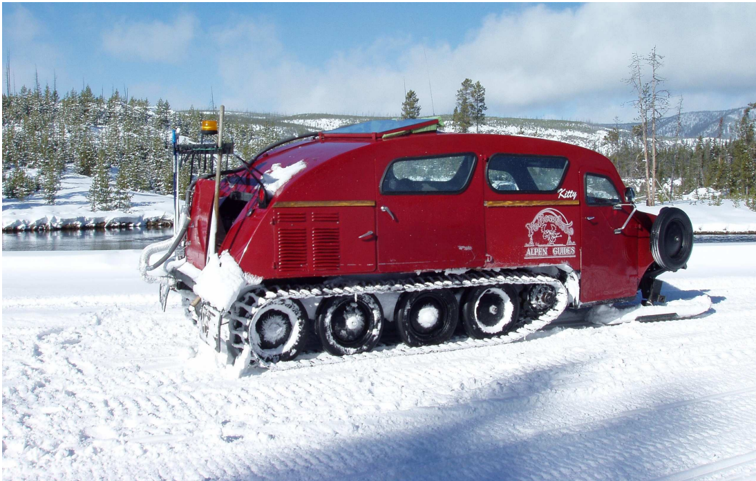
Figure 4. Vintage Bombardier that utilizes a rear engine, forward driven twin track and twin steering ski arrangement. The sample and data lines enter the cabin through a rear roof hatch.
