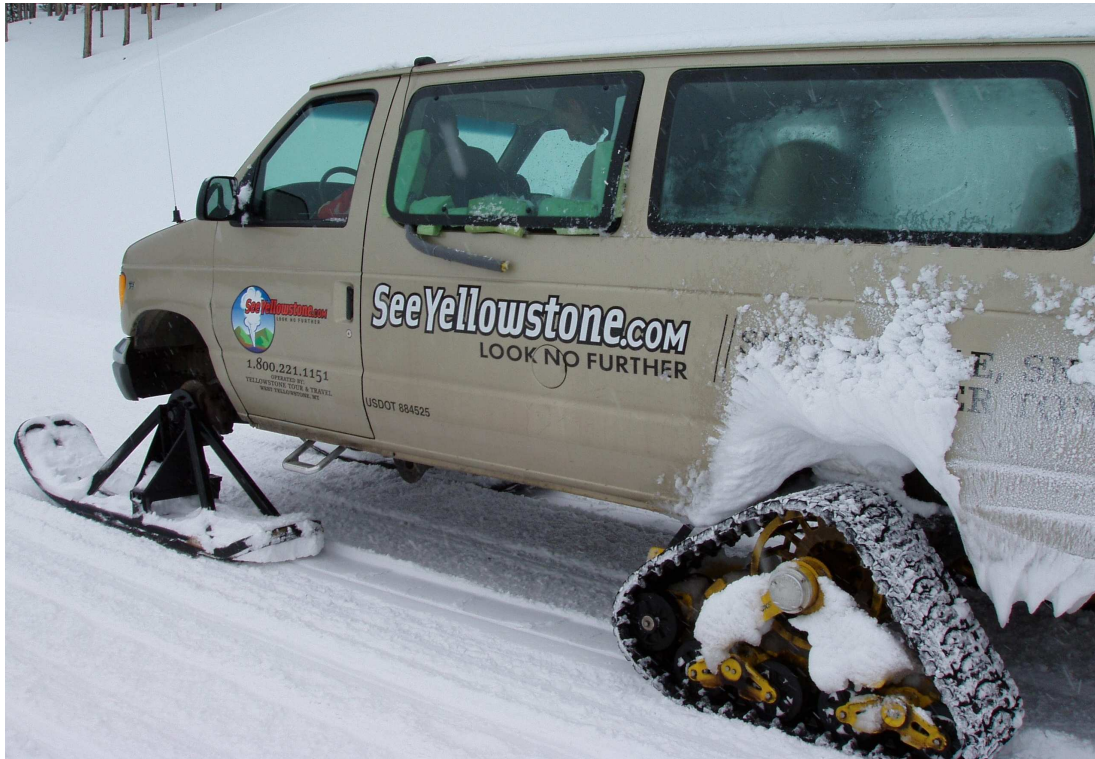
Figure 6. A 2000 Ford Van with a rear driven Mat-trax and ski conversion. Visible is the exhaust exit line.
