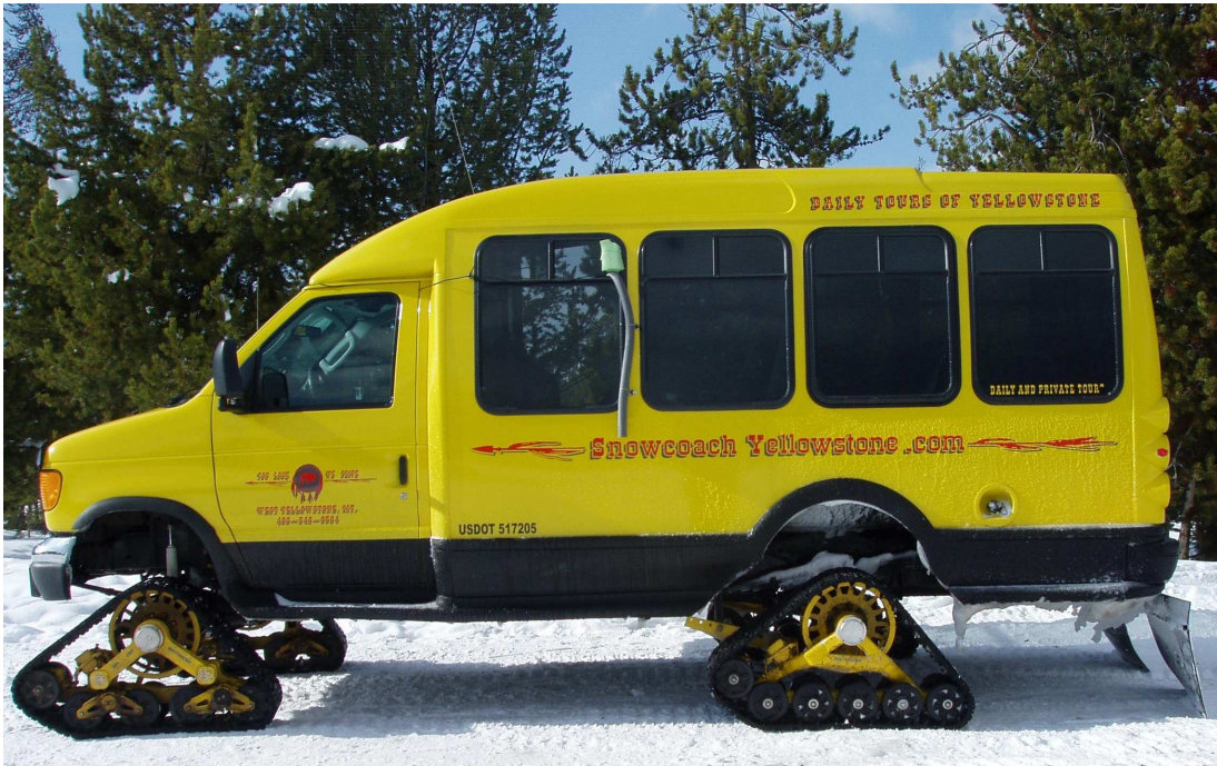
Figure 8. A 2004 Ford VanTerra conversion coach with a 4 wheel drive Mat-trax conversion. Visible is the insulated exhaust exit line.
