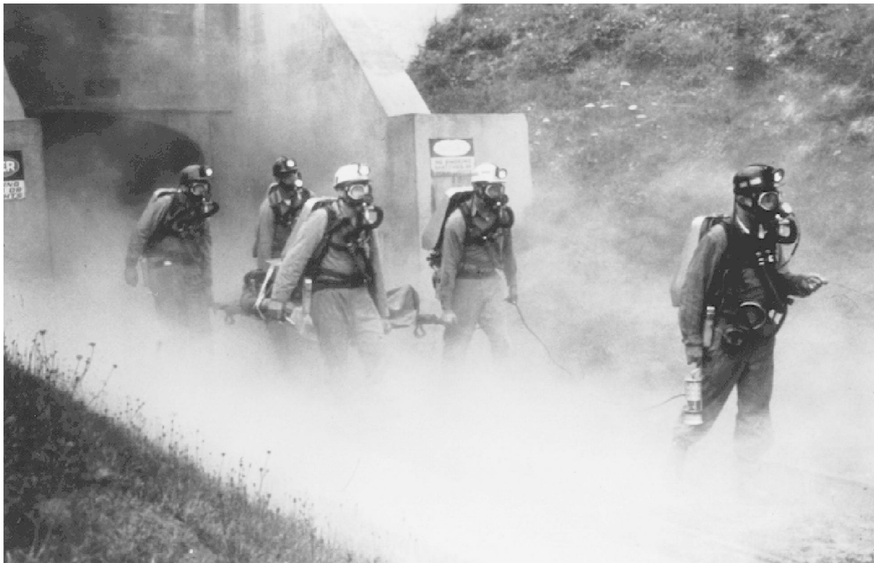
The emergency breathing devices, being tested here, were developed by the U.S. Bureau of Mines, and are used in every underground mine in the Nation. When fires, explosions, and other emergencies occur, these devices allow miners to escape oxygen-poor or smoke-filled tunnels.
