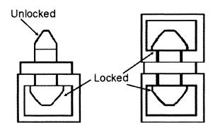
Figure 2—Interbox Connections (Source: Ex. 11-6H)
