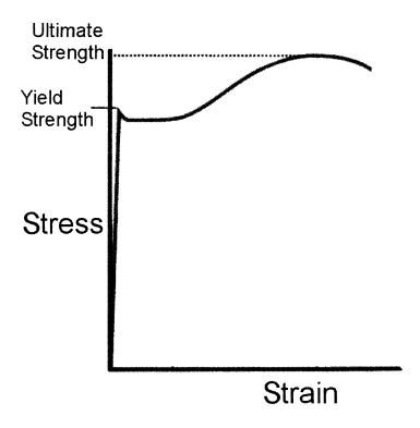
Figure 4—Stress Strain Curve for Steel
