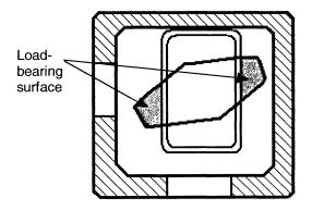
Figure 3—Load-bearing Surface of Interbox Connection (Source: Ex. 41)
