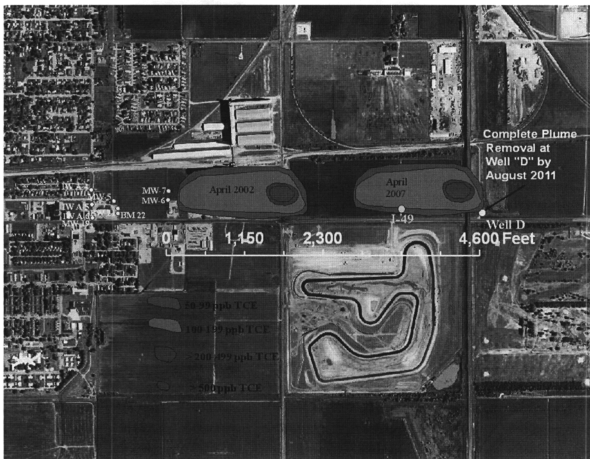
Figure 10. Conceptual model showing downgradient position of North Landfill TCE plume delineated in April 2002.
