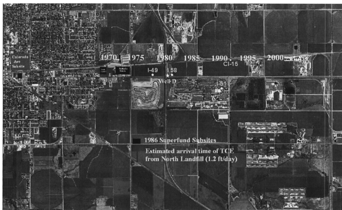
Figure 8. Downgradient high capacity irrigation wells and estimated TCE arrival times in the shallow zone from the North Landfill.
