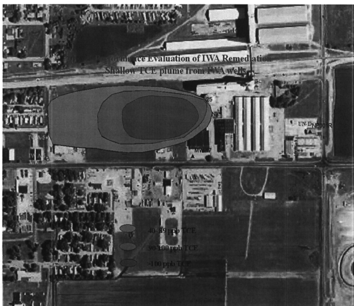
Figure 5. Shallow groundwater TCE plume in December 2006.
