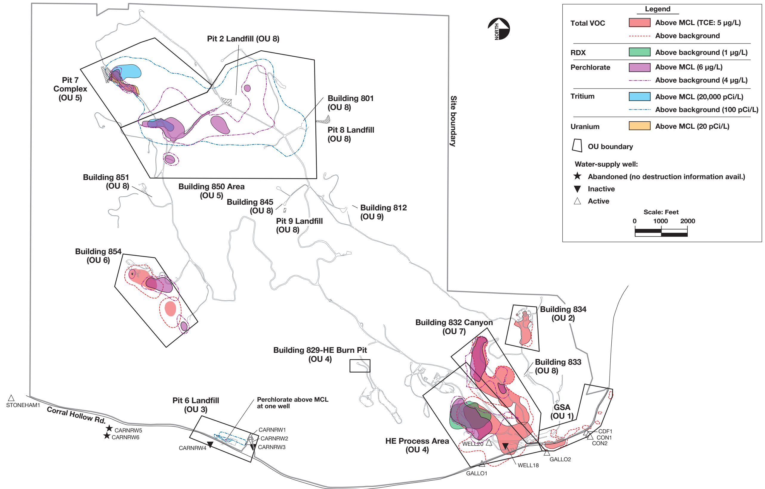
Figure 2.4-2. Map of Site 300 showing operable units with ground water plume outlines and water-supply wells.
