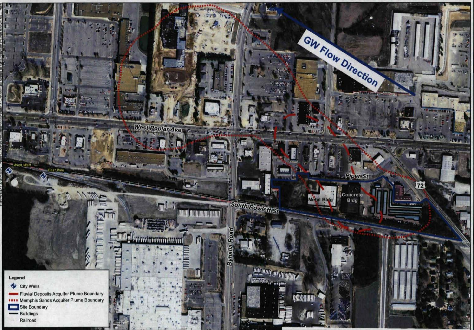
Conceptual Model of Ground Water Plume Above Maximum Contaminant Level (MCL) Smalley-Piper Superfund Site Aerial (Plan) View Collierville, Shelby County, Tennessee
