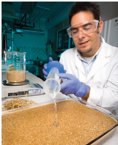
Technician John Michael Henderson combines dilute sulfuric acid with ground wheat straw as a pretreatment. The wheat straw is then autoclaved and transferred to a bioreactor for butanol production.
