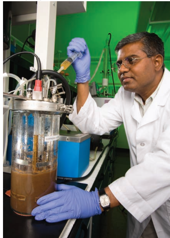
Chemical engineer Nasib Qureshi adds enzymes into a bioreactor to simultaneously hydrolyze wheat straw into simple sugars and produce butanol.
