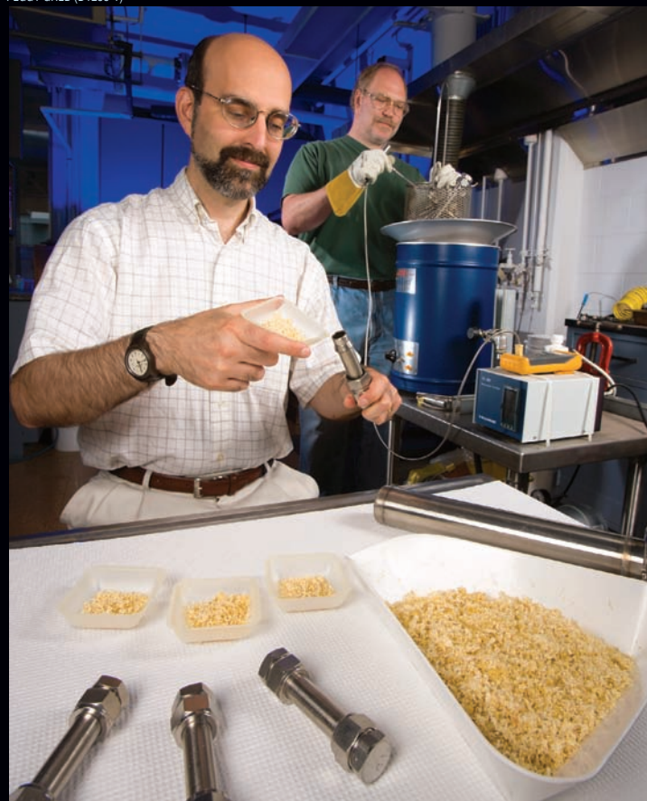
Biochemical engineer Bruce Dien (left) loads reactor vessels with corn fiber while microbiologist Loren Iten lowers samples into a sand bath heater to pretreat for fermentation.
