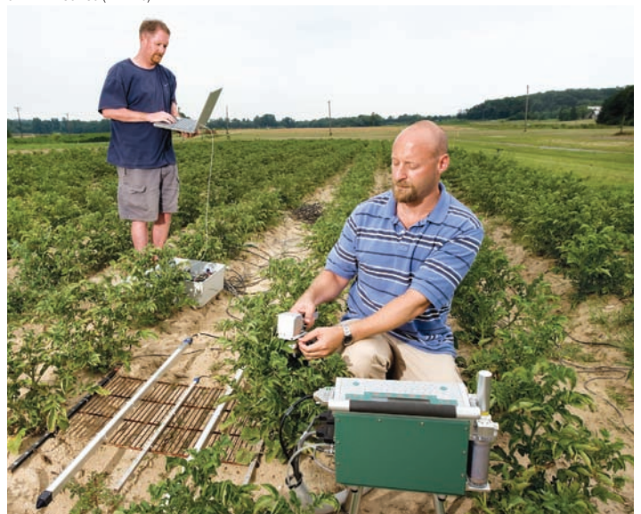
In a Beltsville potato field, engineer Dave Fleischer (right) measures leaf photosynthesis as technician Jackson Fisher downloads lightbar data, which measures light interception in the crop. This information is used to develop models for potato production.
