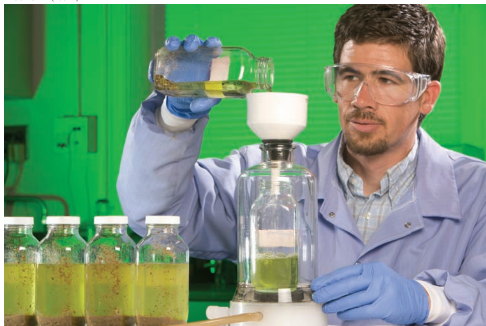
Technician Reuben Anderson filters artichoke extracts in preparation for determination of residues of methiocarb, a molluscicide for slug control.
