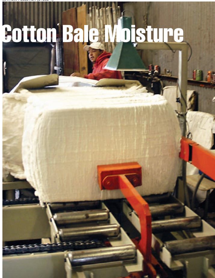
Pilot testing in a commercial cotton gin of a new ARS experimental microwave moisture sensor.
