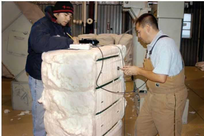
ARS technicians Jimmy Castro (left) and Chris Olmos test industry-standard hand-held probes for accuracy. The problem with these widely used sensors is their inability to determine moisture content deep within cotton bales.
