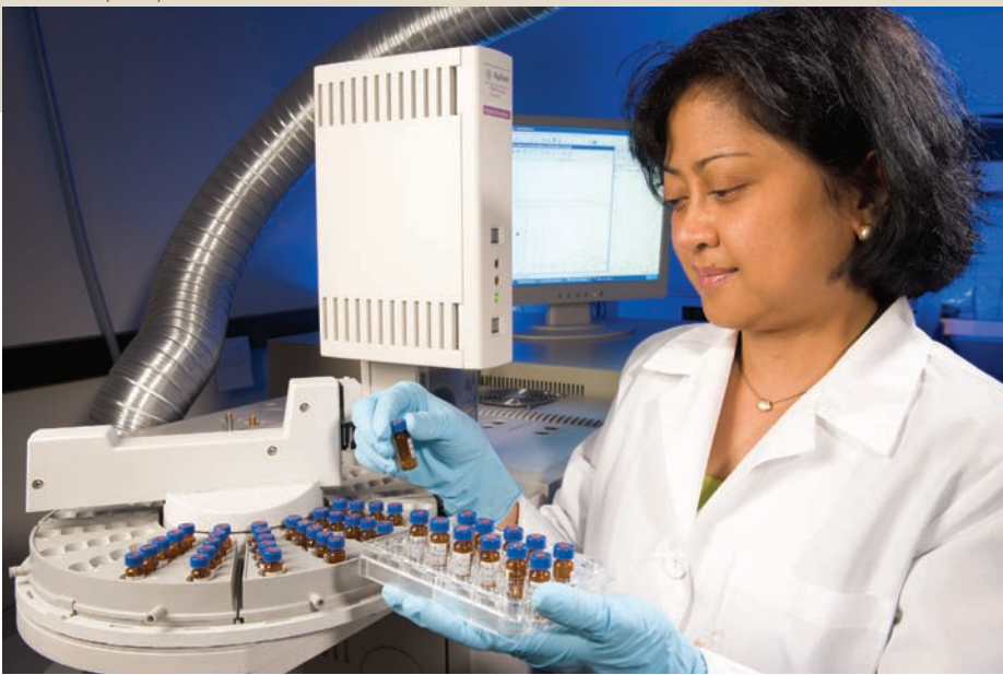
Using gas chromatography/mass spectrometry, chemist Agnes Rimando analyzes pterostilbene content in blueberries.
