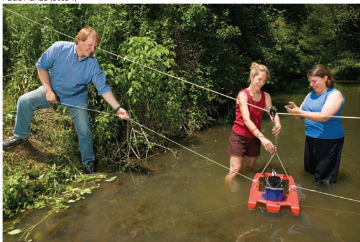
ARS soil scientist Greg McCarty, University of Maryland support scientist Anne Gustafson (center) and ARS chemist Cathleen Hapeman use an Acoustic Doppler Channel Profiler to assess water velocity and channel geometry of a Choptank Watershed stream.
