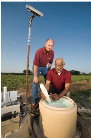
During studies to develop better management practices to reduce or prevent nutrient losses from agricultural fields, University of Maryland associate professor Arthur Allen (kneeling) and ARS soil scientist Ray Bryant collect water quality samples from an automated sampler.
