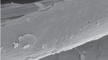
Scanning electron micrographs of untreated wool fiber (top) and wool fiber treated by the ARS biopolishing, shrinkproofing method (bottom). Magnified about 2,500x.
