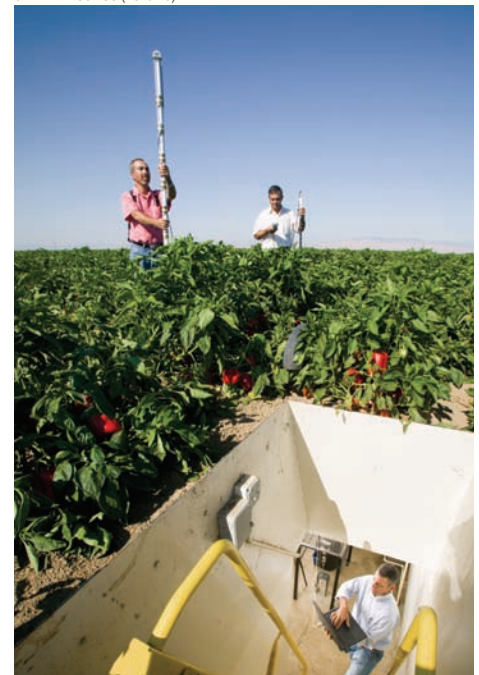
In California's San Joaquin Valley, visiting soil scientist Ron Seligman from Rehovot, Israel, collects data underground inside a lysimeter while visiting engineer Nedal Katbeh-Bader of Hebron in the Palestinian Authority (left) and visiting soil and water scientist Naem Mazahrih of Ajloun, Jordan, place equipment to compare accuracy of soil-water sensors.
