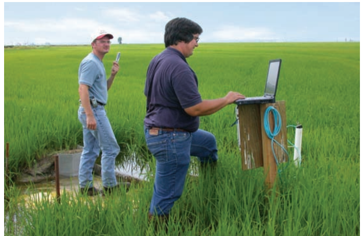
In studies of water use, runoff, and water quality, ARS agricultural engineer Earl Vories (right) and University of Arkansas technician Shawn Lancaster collect data from a MIRI system.
