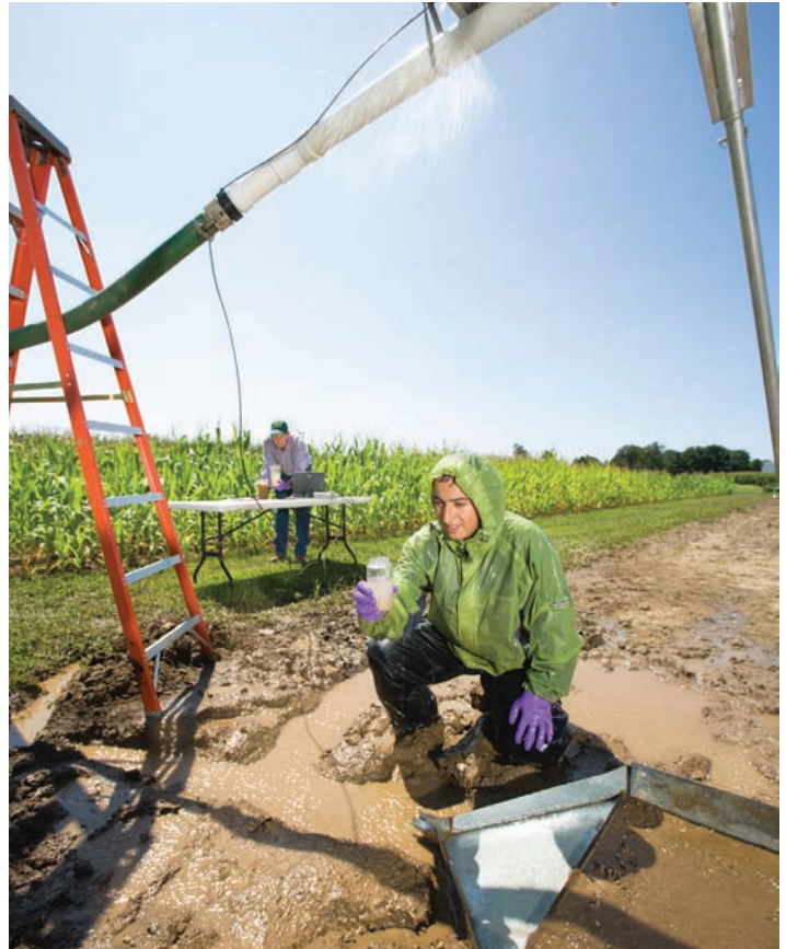
Junior Cesar Avanzi, visiting scientist from the Federal University of Lavras, Brazil, collects sediment to assess the level of erosion control from the use of gypsum-polyacrylamide (PAM) pellets. In the background, Darrell Norton controls the rainfall simulator.
