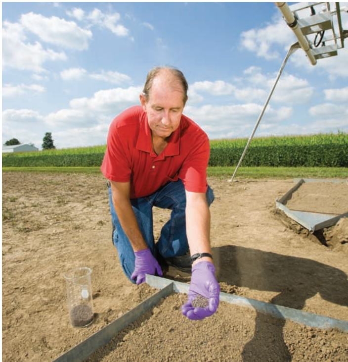
Soil scientist Darrell Norton applies pelletized gypsum and polyacrylamide (PAM) to a soil surface to control erosion prior to a rainfall-simulation test.
