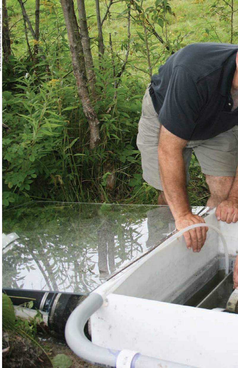
ARS agricultural engineer Kevin King (right) and soil scientist Jim Balogh, of Spectrum Research, Inc., inspect a filter cartridge system being evaluated at a golf course tile drainage site. The cartridge system was donated by cooperating industry KriStar Enterprises, Inc.
