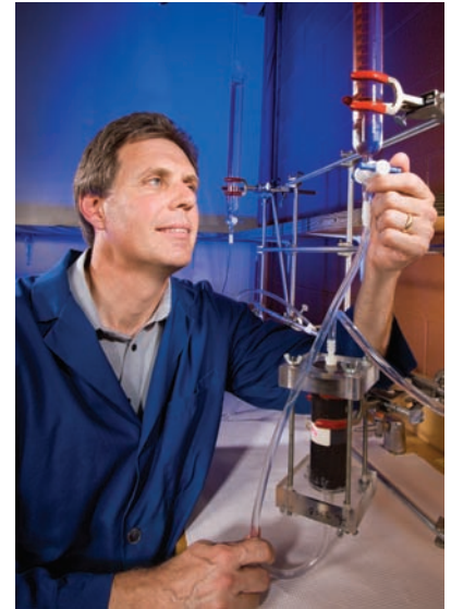
Agricultural engineer Barry Allred conducts an experiment to measure permeability (water flow capacity) of a filter material.
