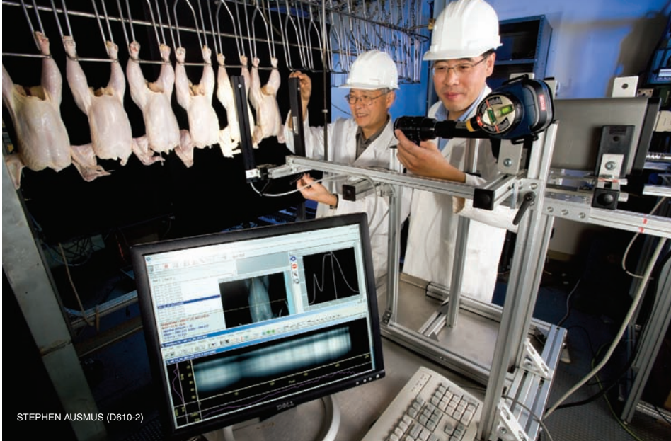
Agricultural engineers Yud-Ren Chen (left) and Kevin Chao make adjustments to a prototype line-scan multispectral imaging system for food safety inspection of chickens.
