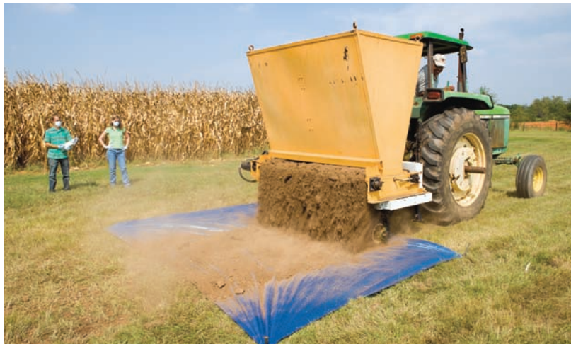
Technicians Stephen Norris and Robin Woodroof observe an application of poultry litter on a tarp used in catching and measuring output for calibration of the precision poultry litter applicator.
