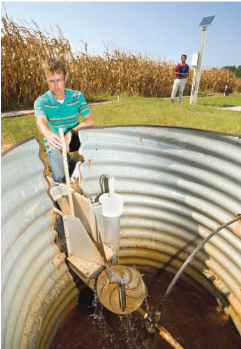
Stephen Norris (foreground) and Dinku Endale calibrate a 6-inch flume and subsampling system used for determining runoff and sediment loss.
