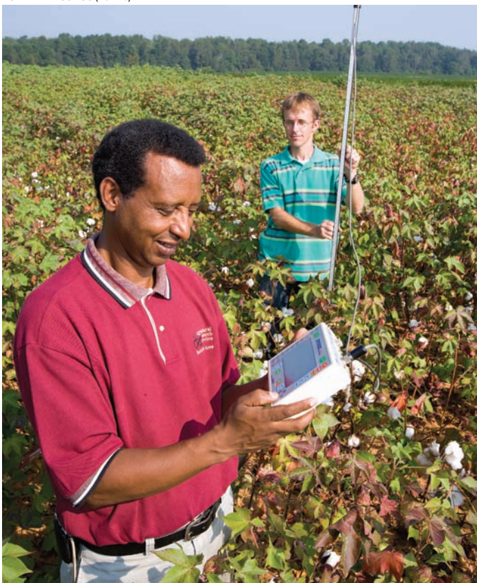
In a conventionally tilled field near Watkinsville, Georgia, agricultural engineer Dinku Endale (foreground) and technician Stephen Norris use a capacitance probe to measure soil water.
