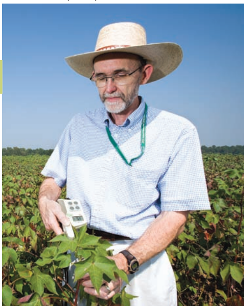
Agroecologist Harry Schomberg uses a chlorophyll meter to determine leaf color before collecting cotton plants for evaluating plant growth and nutrient uptake.
