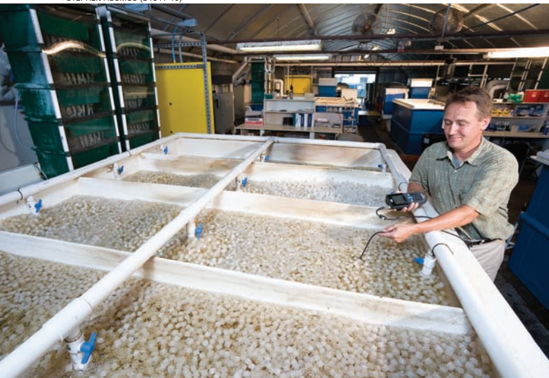
Agricultural engineer Timothy Pfeiffer uses a hand-held meter to measure water quality in a moving bed biofilter.
