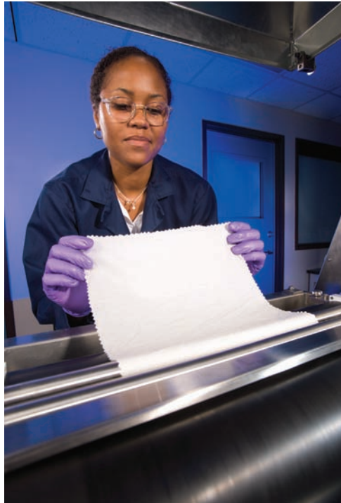
Chemist Nicolette Prevost treats cotton fabrics with a chitosan formulation, which is designed to confer blood-clotting and antibacterial properties on wound dressings and specialty garments.
