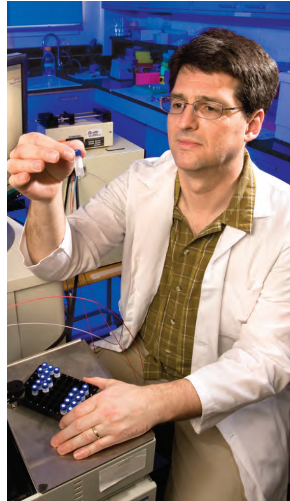
John Lippolis uses a tandem mass spectrometer, which collects the data necessary for proteomics.
