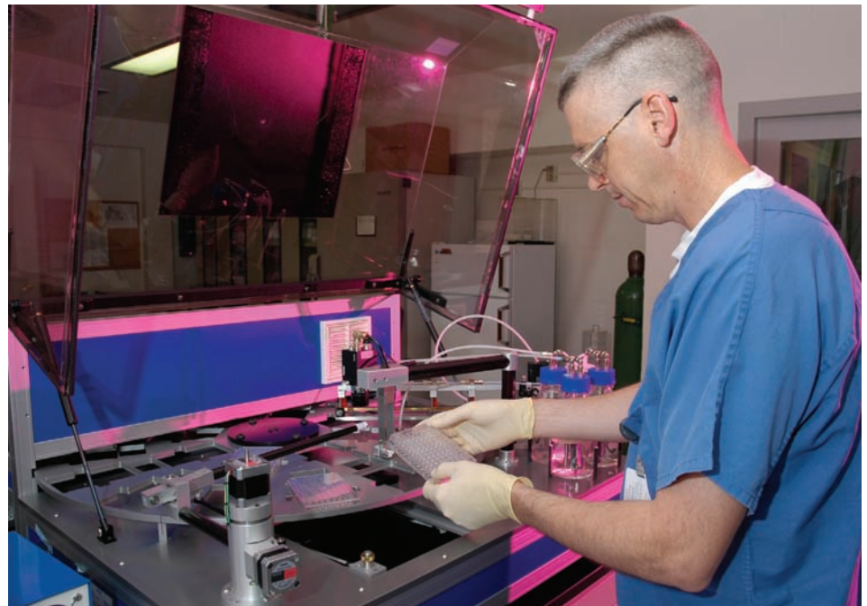
In preparation for sequencing Leptospira ’s genome, technician Rick Hornsby loads a 96-well plate into a machine known as a “colony picker.”
