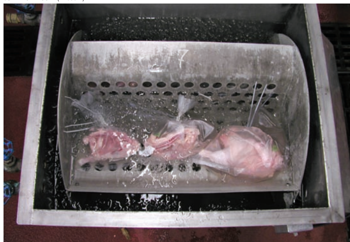
Simulated immersion chilling using a technique of individually bagging broiler carcasses. The bagging prevents bacterial cross-contamination from one carcass to another.
