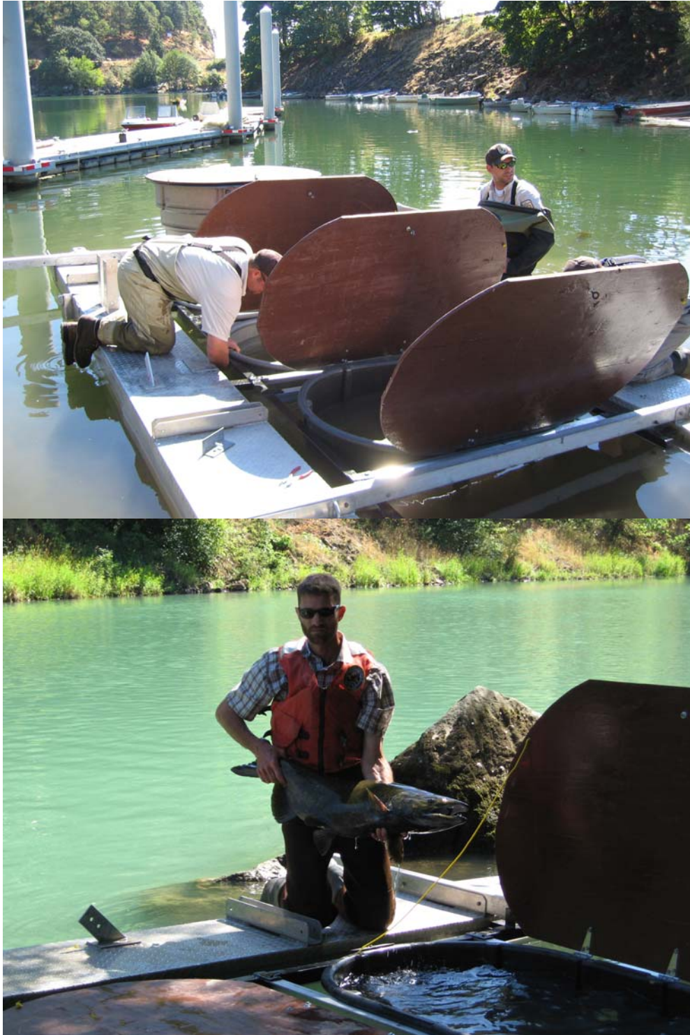
Figure 5. Staging barge constructed for the holding of captured Lower Columbia River fall Chinook salmon in the lower White Salmon River during 2008. The frame and floating pontoons were modified from a rotary screw trap. Three 150-gallon totes were submerged and 10 -3” holes were placed in each tote for water exchange. Two additional totes were mounted to each side of the barge to allow for fish processing determining hatchery or natural origin fish, and to contain anesthesia for affixing radio tags. Lids were placed on totes to provide shade, protection and to prevent escape. Barge constructed by John Meduna, Spring Creek NFH.
