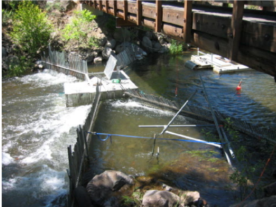
Figure 5. Picket weir at rkm 1 on Shitike Creek. Downstream live box is pictured with the top opened for removal of fish.
