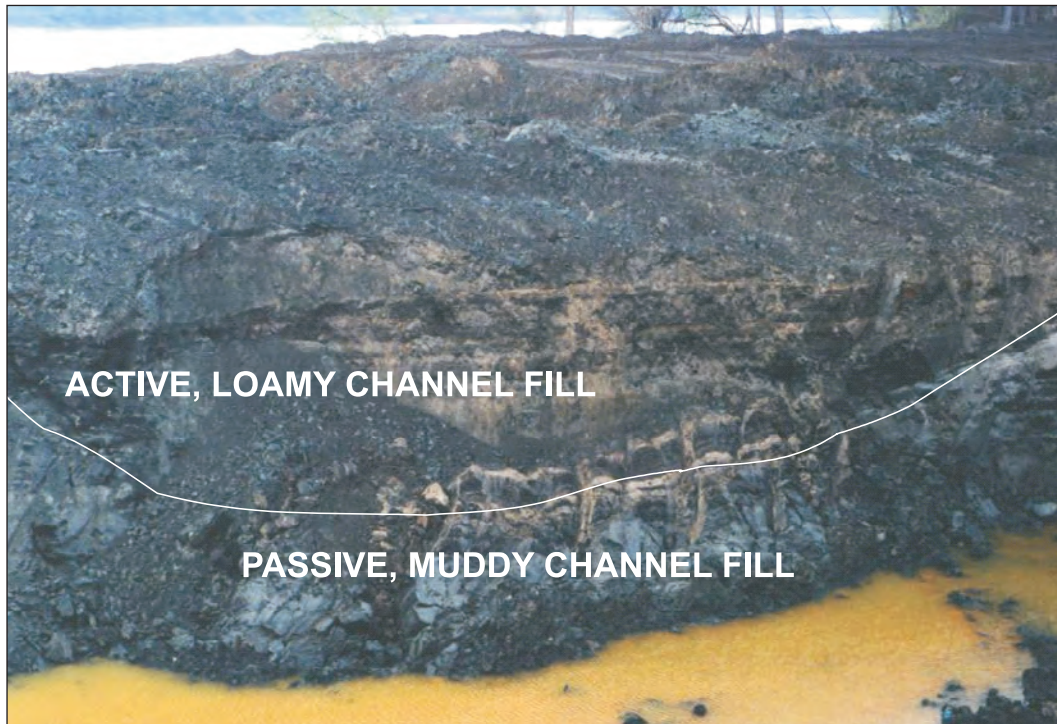
Figure 7. Cross section of a typical channel fill. This cross section was cut at the west end of the excavated chute channel and records the channel drilled in boreholes 50 and 51, cross section B–B'. Height of the bank is about 4 m.
