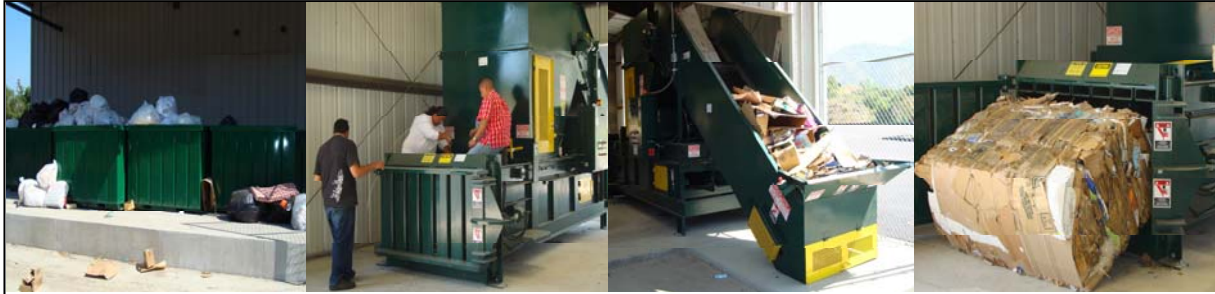
Left & left center: storage containers for recyclable items prior to baling and employees ready the baler for use; Right & right center: cardboard baler; Bottom: cardboard being baled and finished product; Pala Band of Mission Indians, Pala, CA
