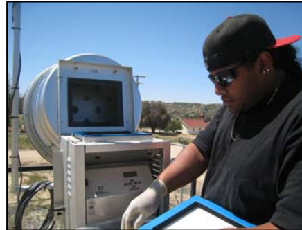
Campo EPA Air Technician changes filter on the PM 10 monitor near Tribal Offices, Campo Band of the Kumeyaay Nation, Campo, CA
