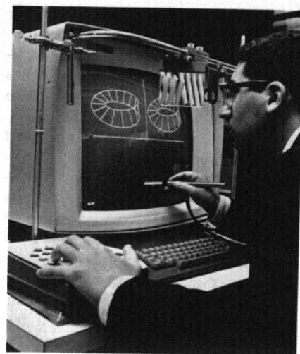
This computer is creating pictures that can be seen with a third dimension—depth. The pictures generated on the screen by the computer have only the dimensions of height and width, but when viewed through the stereoscope mounted in front of the screen they merge into a single, realistically three-dimensional figure. (Photo Brown University)
