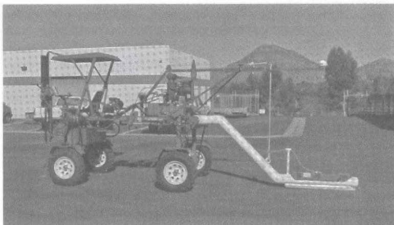
FIGURE 2.4 Mobile dual-dipole electromagnetic induction equipment developed at the United States Salinity Laboratory. (From Corwin, D.L., and Lesch, S.M., Comput. Electron. Agric. , 46, 11–43, 2005a. With permission.)
