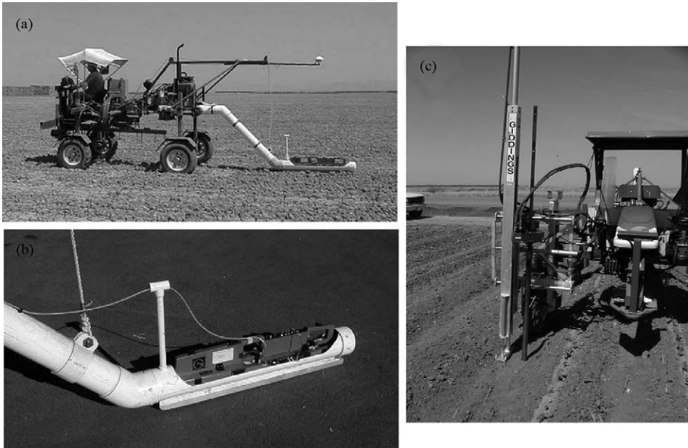
Fig. 1. Mobile EM equipment: (a) complete rig; (b) close-up of sled holding the Geonics dual-dipole EM-38 soil electrical conductivity meter; (c) close-up of Giddings soil core sampler.
