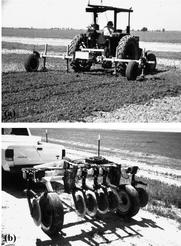
Fig. 4. Mobile ER equipment developed (a) by Rhoades (1992, 1993) and Carter et al. (1993) and (b) Veris Technologies' commercial equipment.
