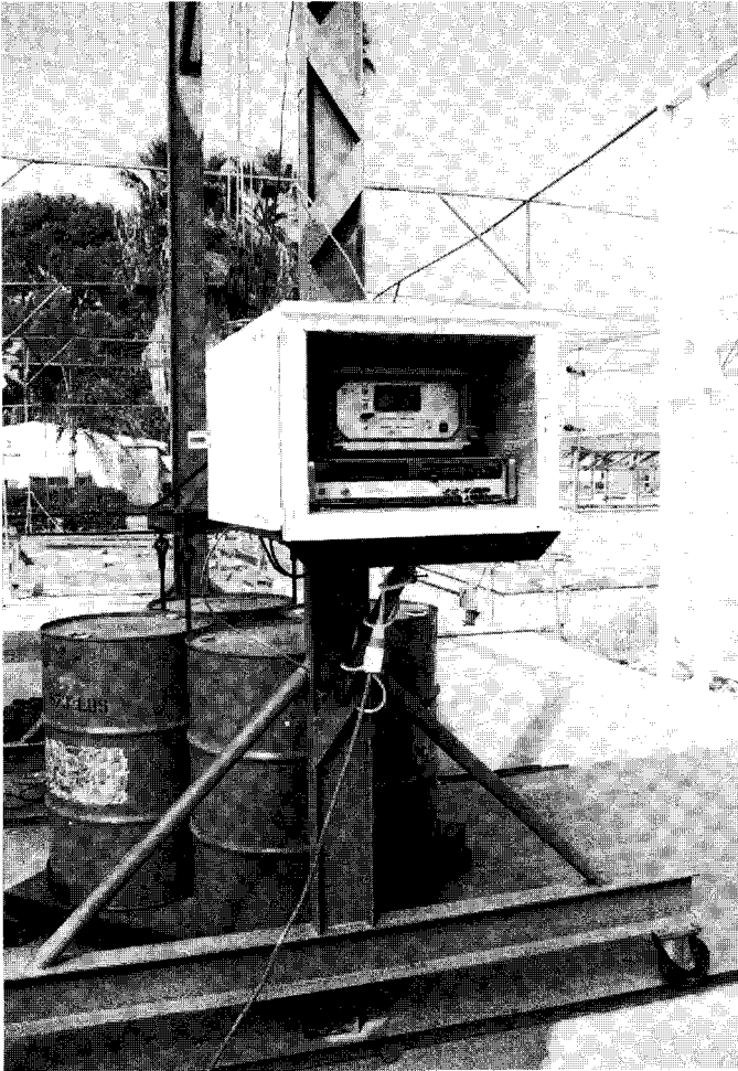
Fig. 9. Encased millivolt meters used to read the load cell
