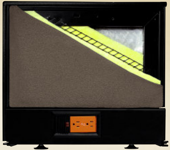
The steel frame and expanded metal skeleton of a Classic XXI panel core enclose acoustic barriers of fiberglass and aluminum foil for a combination of privacy and strength.
