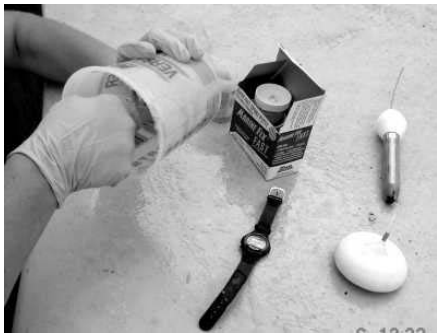
Figure 1: Put all contents from both containers (A and B) in one box of Marine Fix® Fast (MFF). Stir and mix thoroughly for 1.5 minutes.
