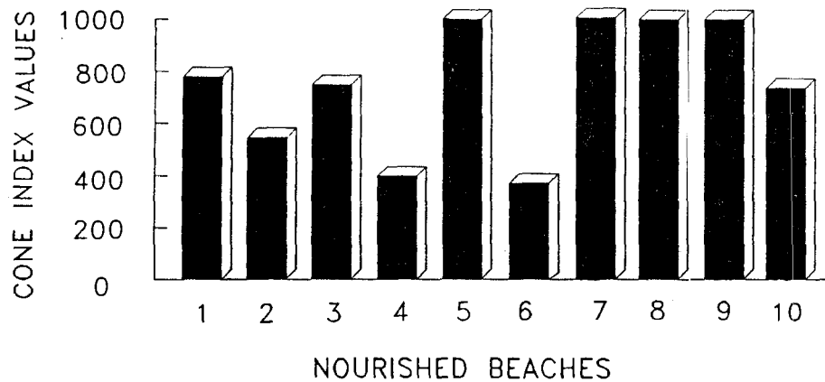
Figure 1. Shear resistance measurements in cone index values at the depth interval 12 inches below the beach sand surface for the following 10 Florida east coast beaches: 1) Fernandina, 2) Jetty Park, 3) Hutchinson Island, 4) St. Lucie Inlet, 5) Jupiter Island, 6) Boca Raton, 7) Pompano, 8) John U. Lloyd, 9) Haulover, 10) Key Biscayne.
