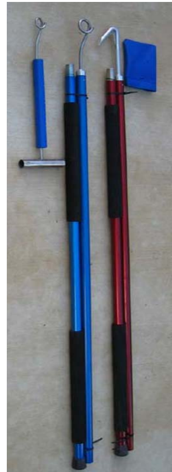
Dehooker kit including from left: turtle dehooker with attached beak block, dehooker and line cutter, © Belldi Consultancy
