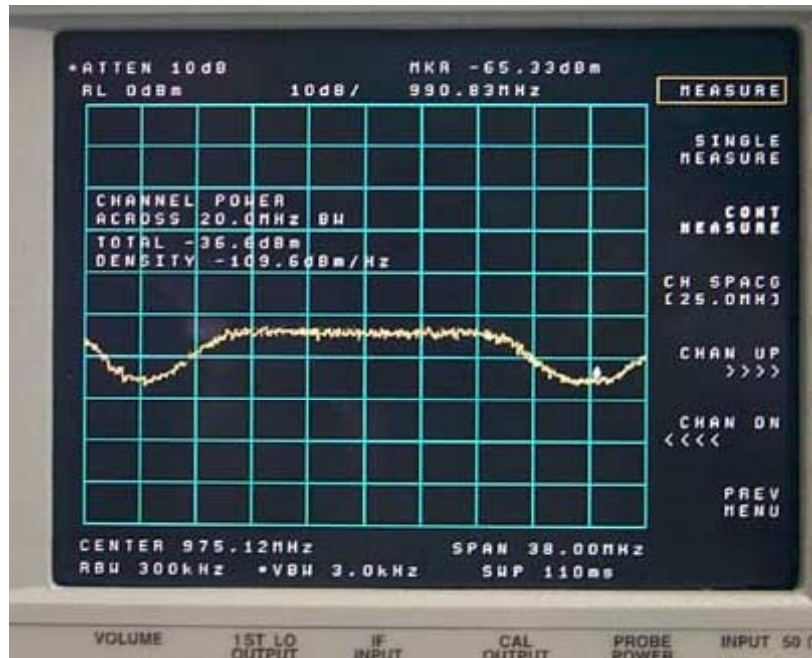
Figure A-9. Single Channel MVDDS IF Interference Plus Adjacent Channels Generated from Arbitrary Waveform Synthesizers
