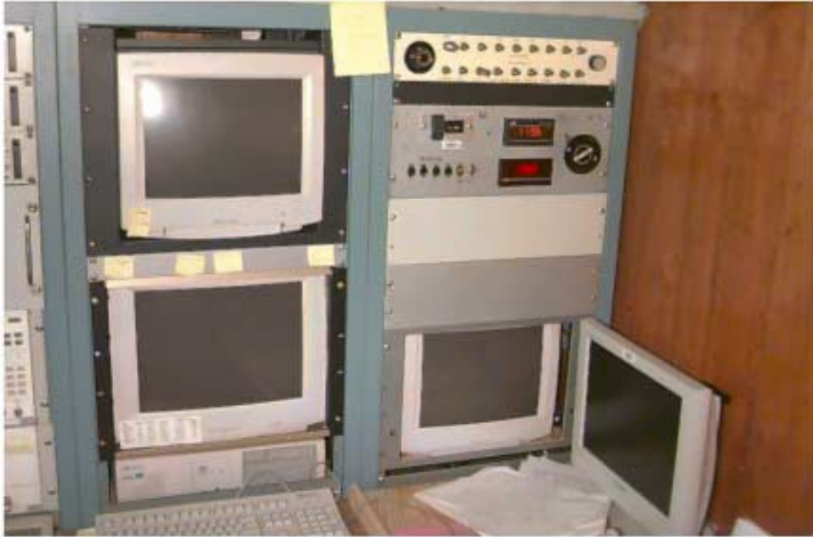
Photo F-4. Port Half of Equipment Rack Showing Data Collection Computer, Picture Displays, and Genset and Antenna Controls
