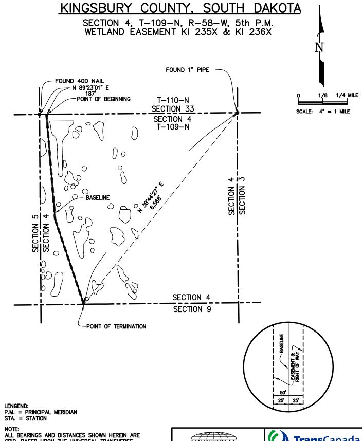
ALL BEARINGS AND DISTANCES SHOWN HEREIN ARE GRID, BASED UPON THE UNIVERSAL TRANSVERSE MERCATOR (UTM), ZONE 14 NORTH, AS DERIVED FROM A GPS SURVEY, PERFORMED IN MARCH 2006.
