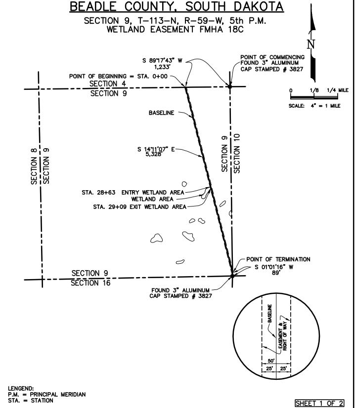
ALL BEARINGS AND DISTANCES SHOWN HEREIN ARE GRID, BASED UPON THE UNIVERSAL TRANSVERSE MERCATOR (UTM), ZONE 14 NORTH, AS DERIVED FROM A GPS SURVEY, PERFORMED IN MARCH 2006.
