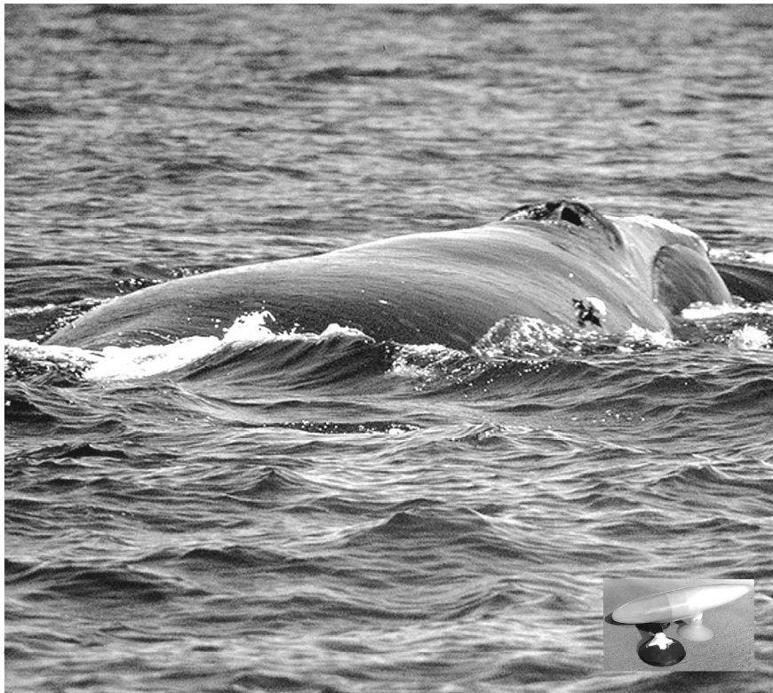
Figure 1. The DTAG encased in a moulded polyethylene fairing attached to a North Atlantic right whale in the Bay of Fundy, August 2000. The inset shows a detailed view of the tag package.
