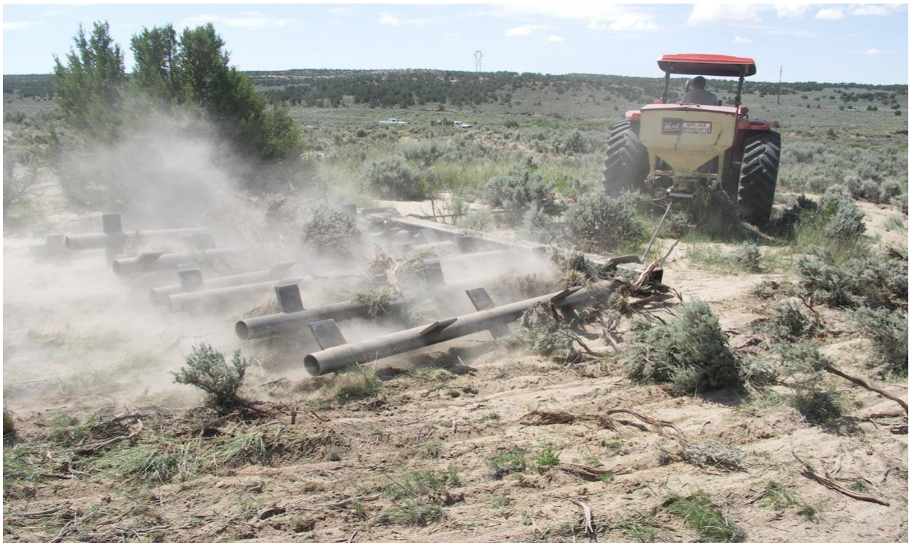
A Dixie Harrow thins sagebrush on BLM land on Crow Mesa while a seed broadcaster on the back of the tractor spreads seeds that will produce grasses and forbs for deer and elk.
