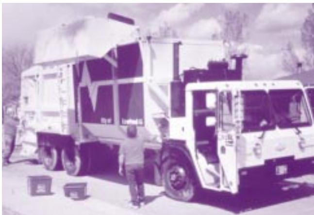
Loveland's semi-automated dual-collection vehicle. Crews put recyclables into the split side-loading compartment and trash into the rear-loading packer compartment.
