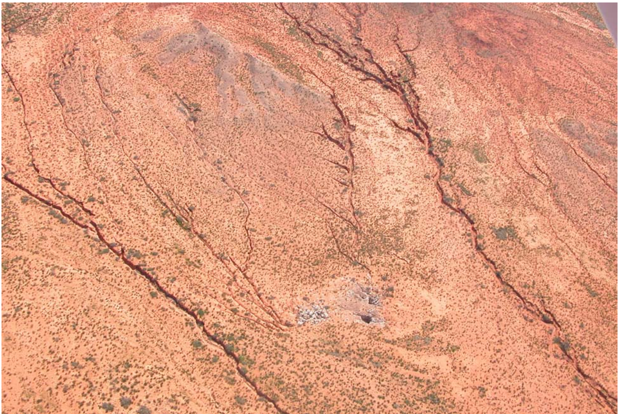
Figure 11. Low-angle aerial photograph of diverted drainage, vanishing streams, and the open sinkholes that capture them, in the Forty-niner Member of the Rustler Formation exposed in Nash Draw, for comparison with Figure 8.
